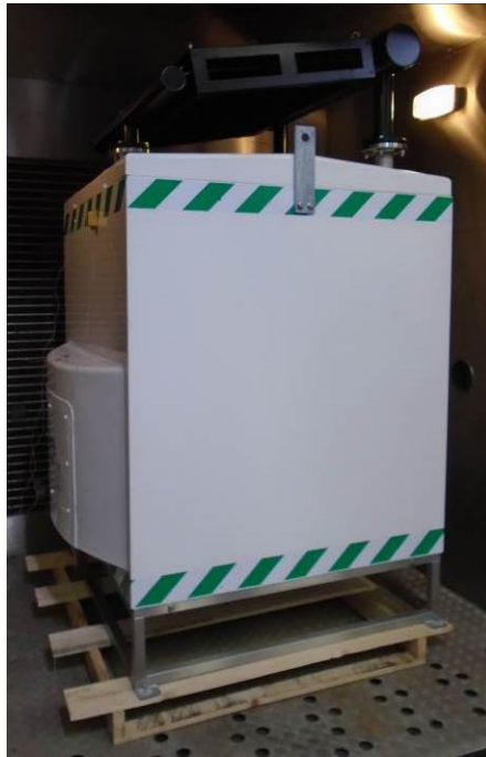
Figure 1.3.1 Passively cooled emergency tank shower as delivered located on wooden pallet without the stretch wrap cover
