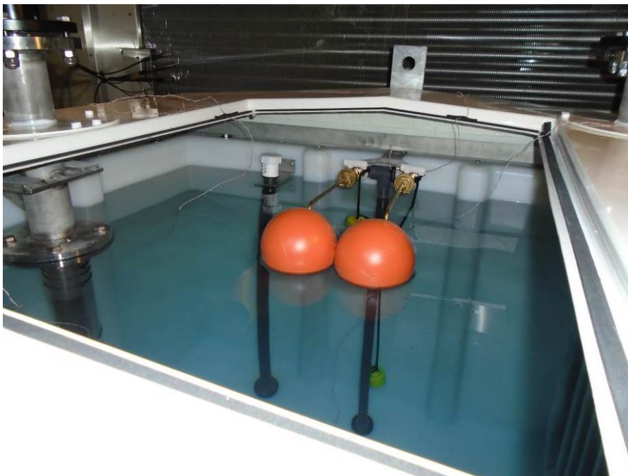
Figure 2.1.8 Shows the passively cooled emergency tank shower filled with water
