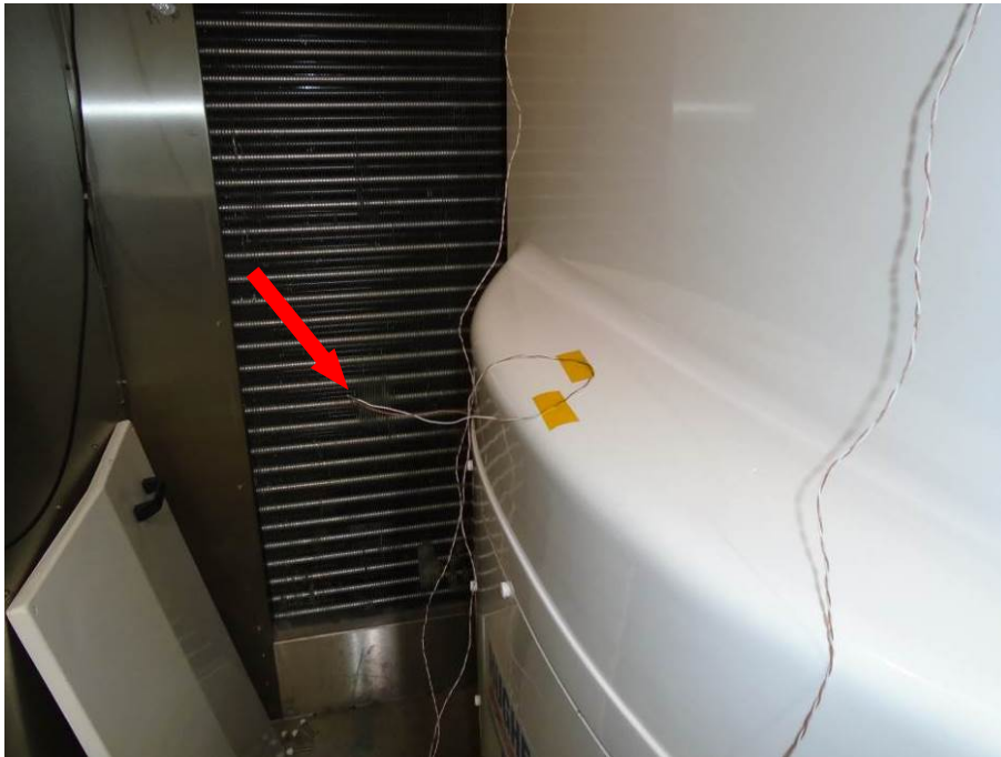
Figure 2.1.7 Local ambient thermocouple (installed by TÜV)
