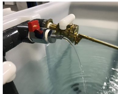
Adjusted setting set to a quicker water dumping rate allowing steady flow of water from the frequency valve
